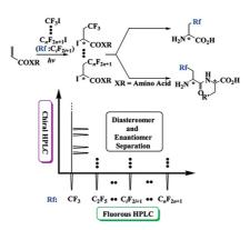
A fluorous racemic mixture synthesis (FRMS) of nonproteinogenic polyfluoro amino acid and peptide precursors was developed by the orthogonal use of fluorous and chiral HPLC columns.
