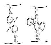
Van der Waals interactions between effector molecules in aqueous solution lead to contraction of polyallymine gel particles, which for benzoic acids increase from about 18% to 70% by the presence of nitro groups, and to 67% with naphthalene derivatives. The observed cooperativity indicates dispersive forces as major driving factor for volume changes in such intelligent materials.
